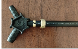
Step 3: Round & Chamfer the pipe (3-5 rotations).
