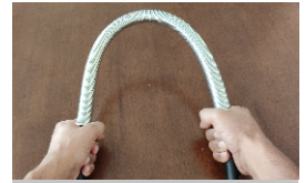
Pipe Bending: Bend pipe using Internal / External bending springs.
