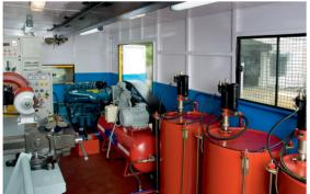
Mobile Service Units are largely classified in to Mobile Lubrication Unit and Mobile Workshop Unit. Mobile Lubrication Unit is equipped with lubrication containers and pumps to pump out the lubricants to service line provided with hose reels and control guns. Mobile Workshop Unit is a vital ancillary at highway breakdowns and construction sites. It is equipped with workbench, welding gensets, battery chargers etc. and equipments for any major or minor repair.
