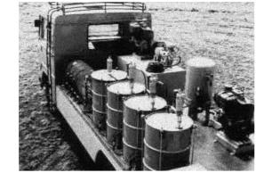
ATS ELGI Mobile service units comprise of servicing equipments like grease pumps, oil pumps, air compressors, hose reels, diesel generating sets, welding equipments, work space, pneumatic tools, control panels, car washers, storage tanks, tool trays, fire extinguishers, tyre inflators, etc.
